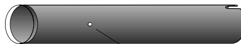
Mark center of hole with punch Drill pilot hole with 1/8 " drill bit Drill pin hole with 3/16" drill bit Install clevis pin and safety
