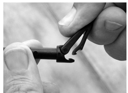
Practice unlocking the latch repeatedly until you can do it without difficulty. Then, practice doing it with your eyes closed. When you are unlocking the latch in order to remove your battens when breaking down your glider, the tip will be hidden from your view below the sail. You will need to be able to unlock the latch easily without having to look at it. Again, the steps in brief are:
